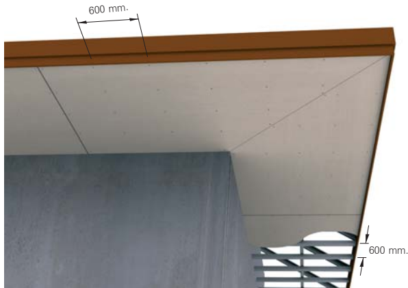
Figure 22 : Board layout for soffit Lining (1)
